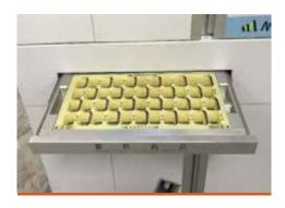
DTA Trays: The two trays, each with 44 compartments, are designed for half and irregularly-shaped drugs, operating alternatively to enhance efficiency. In the case of off-machine drug replenishment, the DTA trays will automatically open, with medication information provided on the screen and replenishment lists printed.
