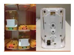
Intelligent Cassettes: Equipped with 348 intelligent cassettes of three types (S, M, and L), avoiding medication blockage with unique dispensing control technology.
