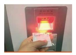
Built-in Barcode Reader: Supports one-dimensional and two-dimensional barcodes, facilitating the process of medication verification.
